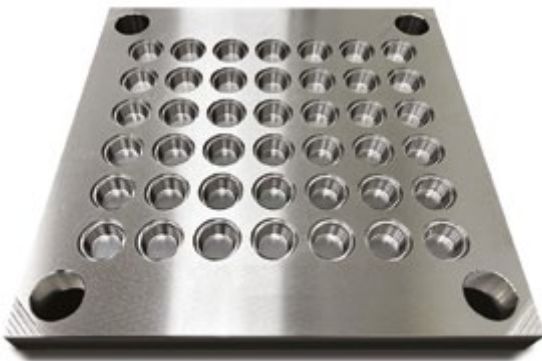
Multicavity mould: ±6µm pitch accuracy in 20 hours machining
