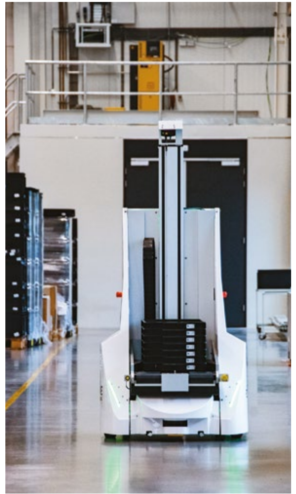
Prodrive uses AGVs for internal logistics automation.
