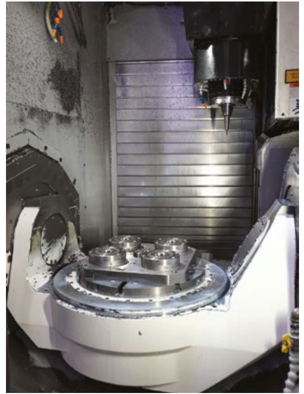
The Makino D500 has a robust construction, making it suitable for heavy-duty 5-axis machining of stainless steel.
