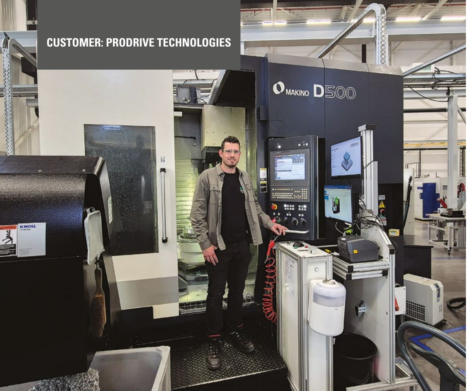
Job Heijlighen in front of one of the 5-axis Makino D500 machining centres.
