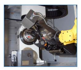
sequence, reduces risk of incorrect load, provides rapid loading of fixtures into the machine, helps with sequential machining, and yields higher productivity and increased efficiency. It lets the operator keep the work-setting station loaded while a part is in the machine, providing increased output at a slightly higher initial cost.
